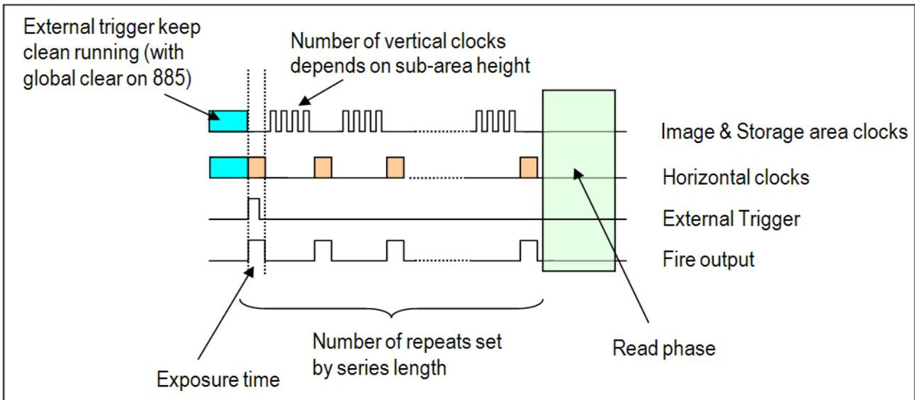
External Start trigger in Fast Kinetics mode
