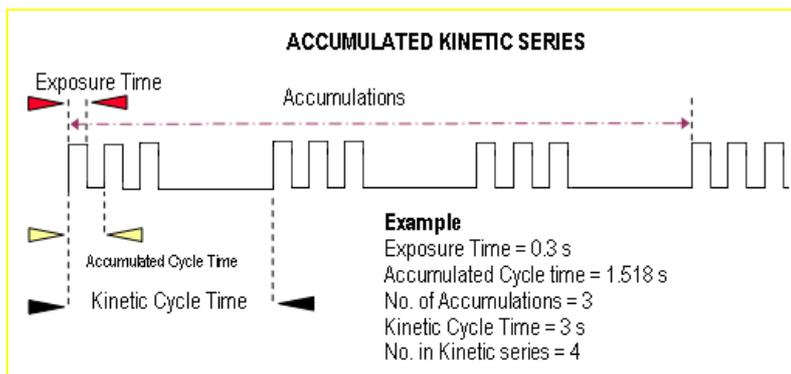
**NOTE:** In External Trigger mode the delay between each scan making up the acquisition is not under the control of the Andor SDK, but is synchronized to an externally generated trigger pulse.
