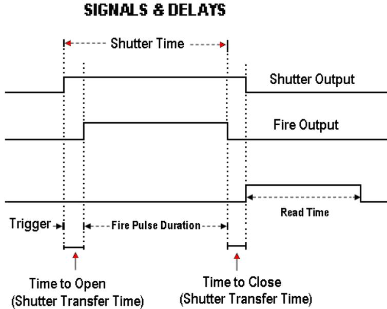
Figure 9: Timing diagram for shutter and fire pulses in internal trigger mode
