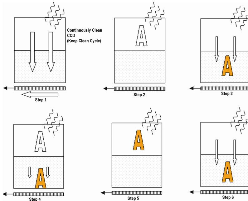
Figure 8: Capture sequence for a Frame Transfer CCD
