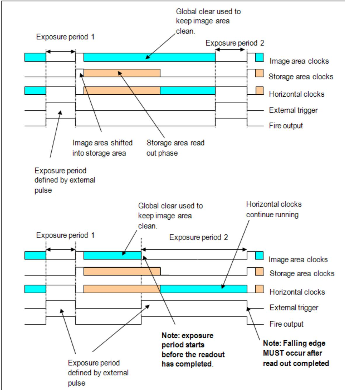
External Exposure Trigger in Frame Transfer mode (885 model only)
