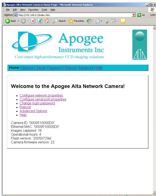
The camera home page contains a snapshot of useful information about the system, including the number of images the system has captured, hours it has been operational, and versions of the internal firmware. This information may assist Apogee's technical support, should you ever require service on your camera system.
