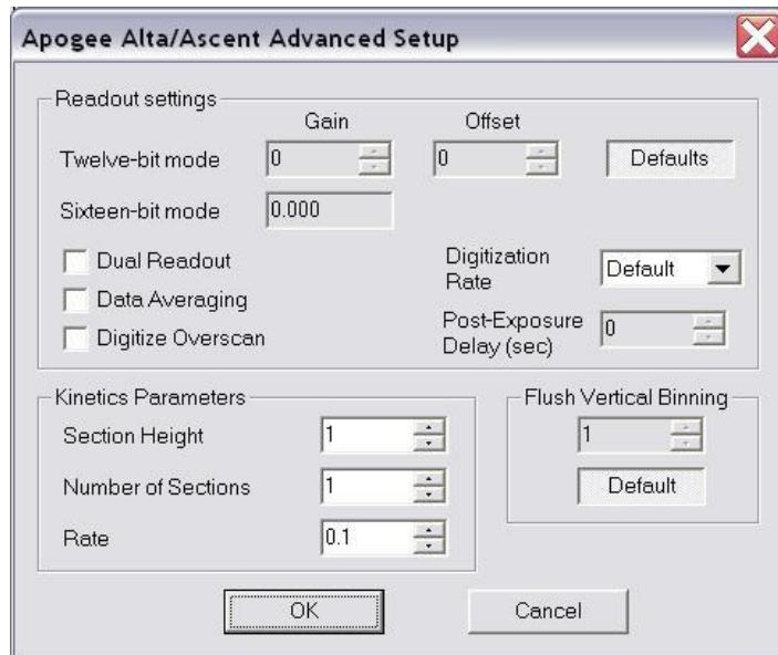
The **Gain** and **Offset** for Twelve-bit digitization mode can be changed from their factory values: you must unclick the **Defaults** button to unlock the edit boxes. The Gain for Sixteen-bit mode is not adjustable, but its value is displayed. You can also indicate whether to **Digitize Overscan** (the part of the CCD sensor surrounding the imaging area which is covered by an opaque mask). In some applications the overscan region is used as part of the calibration process.
