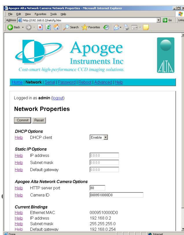
The **Network** page contains the TCP settings for the camera. From this page, the camera can be configured for a static IP network setup. Also on this page, the camera name can be selected (the
