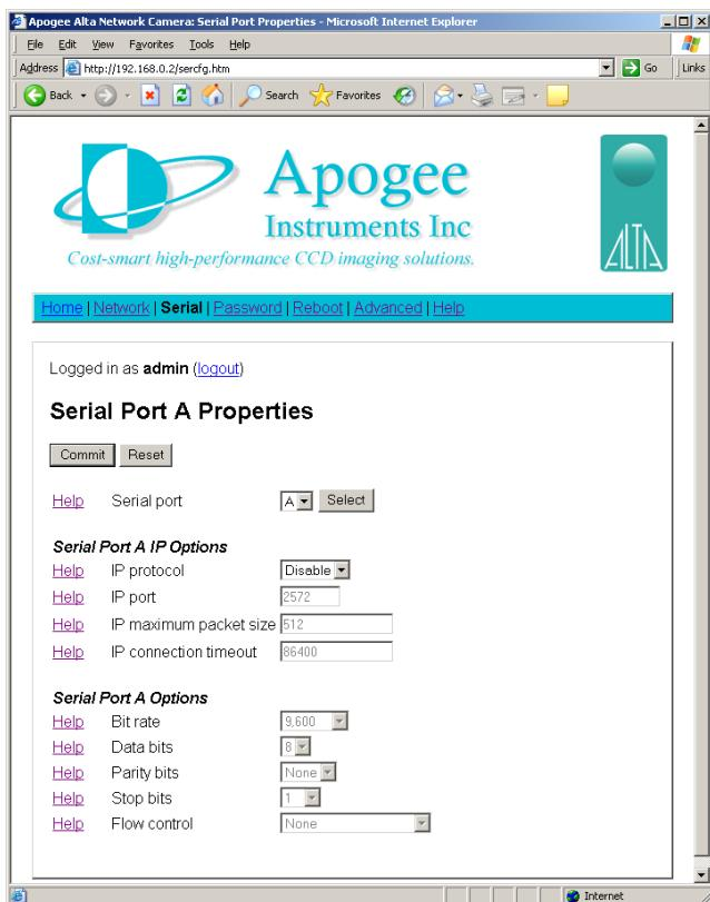
The **Serial** page lists all of the settings related to controlling the camera's on-board serial ports. The user can switch between Serial Port A and Serial Port B by changing the port from the drop down list.
