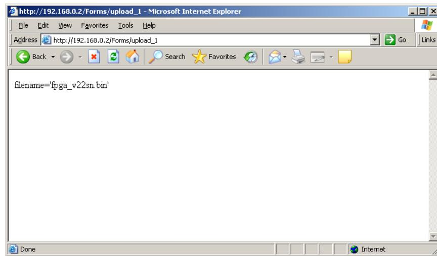
Again, press the browser's **Back** button. Now click the **Write** link in the update firmware section. The camera will send back the final confirmation screen below.
