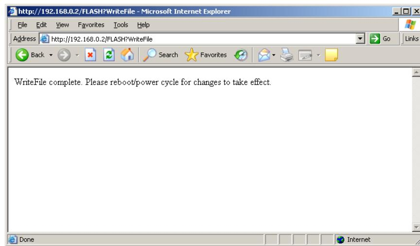
At this point, the new firmware has been loaded into the camera. The camera system should be power cycled for the new update to take effect, and the process will then be complete. On the next power up of the camera, the new firmware will automatically be loaded.
