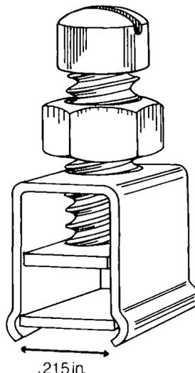
These Surgical stainless steel clamps are used to create selective regional arterial stenosis, specifically, renal ischemia leading to renal hypertension. These clamps are 4mm inside dimension and have a removable throat plate for implantation. Stenosis is accomplished by advancing the movable plate by means of a screw at the back of the clamp. A locking nut is provided to insure against slippage.
