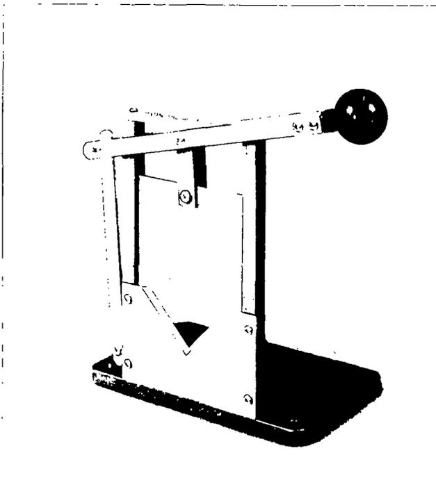
One stroke instantly decapitates rats, mice and other small animals. The blades are hand-honed stainless steel and form an opening  $1\frac{3}{4}$  along each side. All surfaces are accessible to allow washing without disassembly.
