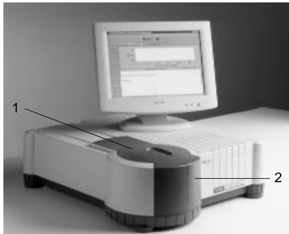
Cary 50 showing the sample compartment lid (1) and front panel (2)
