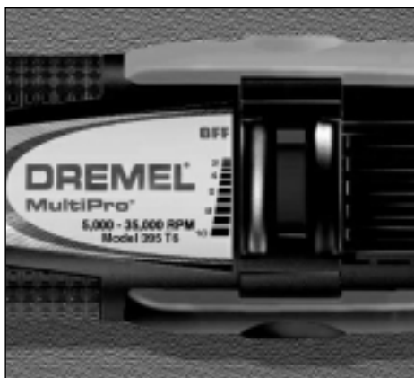
The Settings for Approximate Revolutions Per Minute Rotary Tool Variable Speed Model 395T6.
