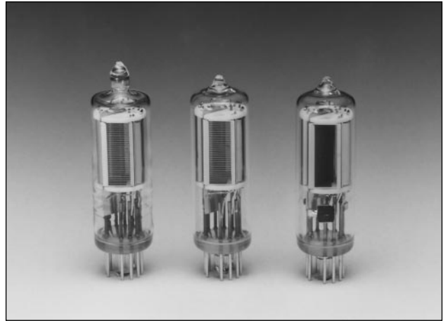
▲ Left: Quartz window Center: UV window Right: Meshless type (R6357)
