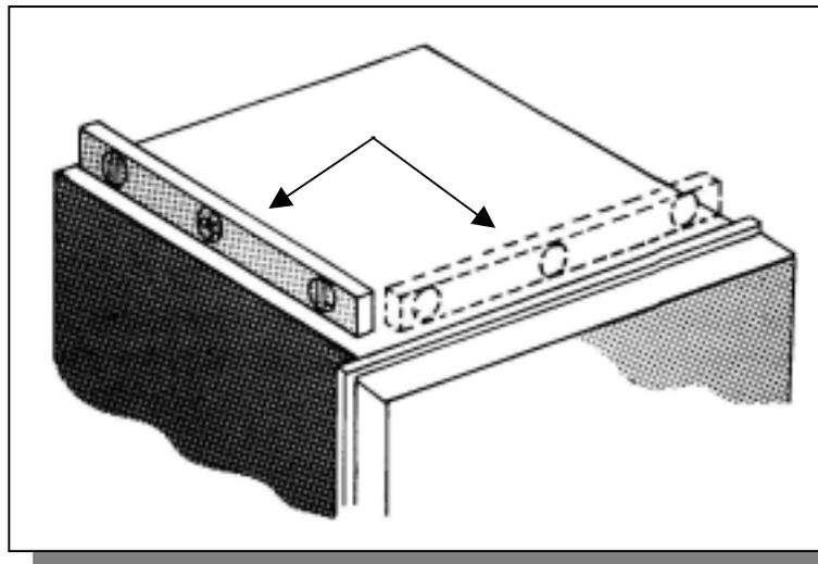
Position the level in both directions to ensure the washer is level front-to-back and side-to-side.
