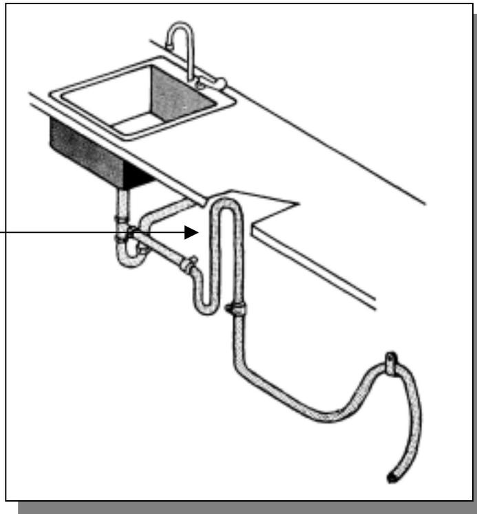
If you route the drain piping to a sink drain and use an air gap, refer to Figure 3-14 for the placement of the air gap.
