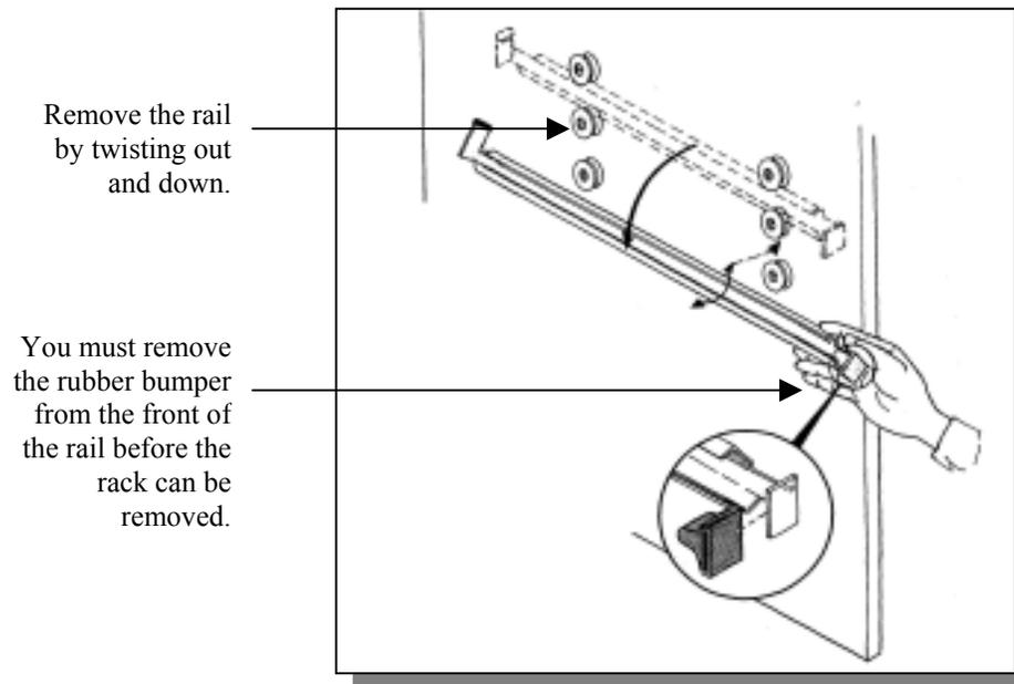
6. Pull the upper rack forward and lift the front until the wheels disengage from the track.
