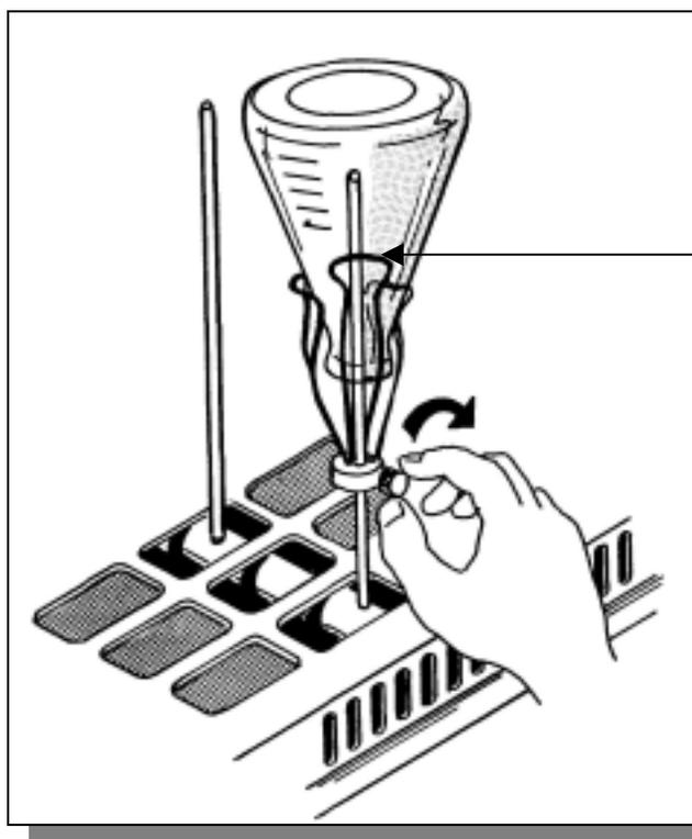
Press the glassware into the glassware holder. Then, turn the set screw counterclockwise to loosen the glassware holder hub. Position the glassware holder so that the spindle is near the center of the glassware. Turn the set screw clockwise to tighten the glassware holder in place.
