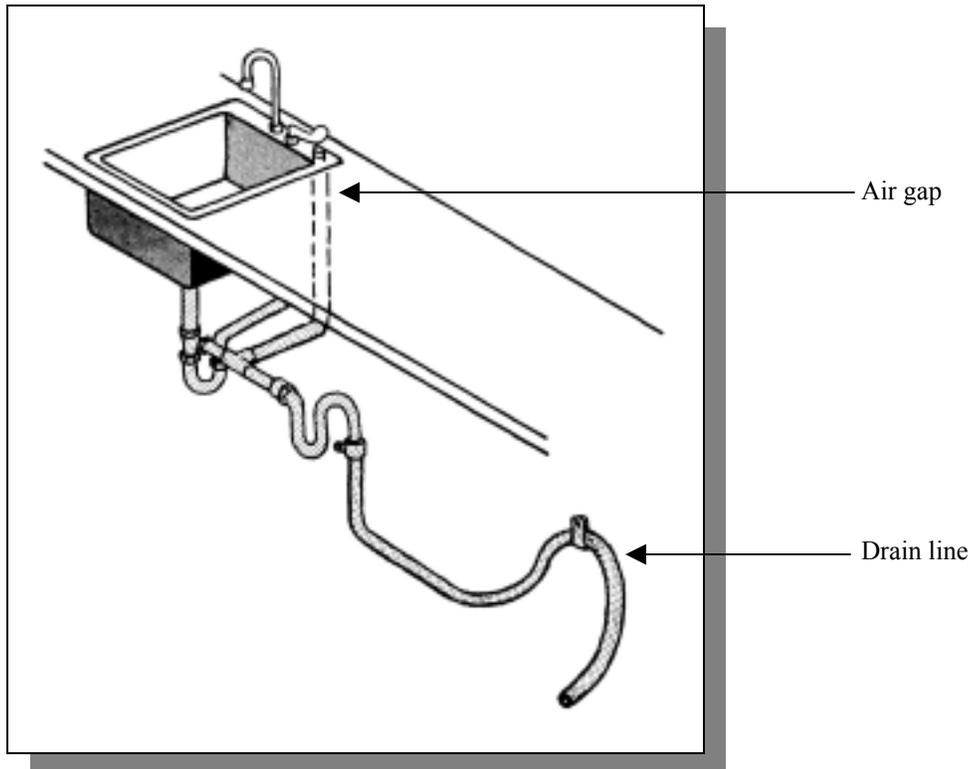
If you route the drain piping to a floor drain, refer to Figure 3-15 for placement of the drain tubing and trap.
