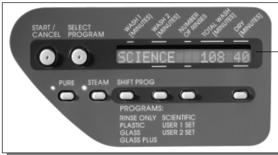
The Scientific wash cycle is selected. The wash will run a total of 108 minutes, with a 40 minute drying time.
