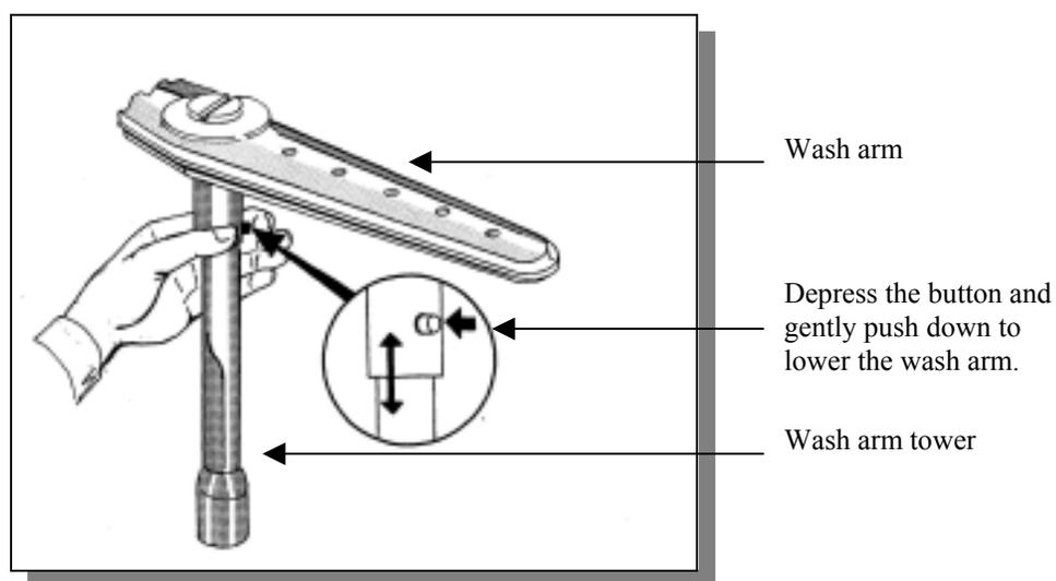
4. Secure the wash arm by clicking the wash arm into the upper hole in the wash arm support tube.
