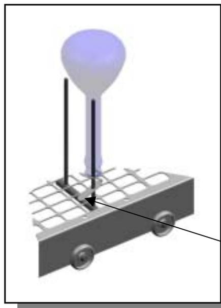
Squeeze the spring clip together and raise or lower the clip to position the glassware properly.
