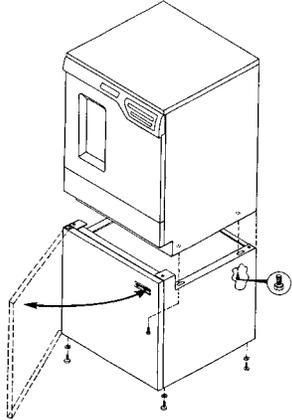
A technical line drawing of a rectangular stand designed for a glassware washer. The stand has a front door that is shown in an open position, indicated by a curved arrow. The washer is mounted on top of the stand. The stand has four legs, each with a small circular detail at the base, possibly representing a leveling foot or a fastener. A small circular detail with a screw symbol is also shown on the right side of the stand, likely indicating a fastener for the front door. |
