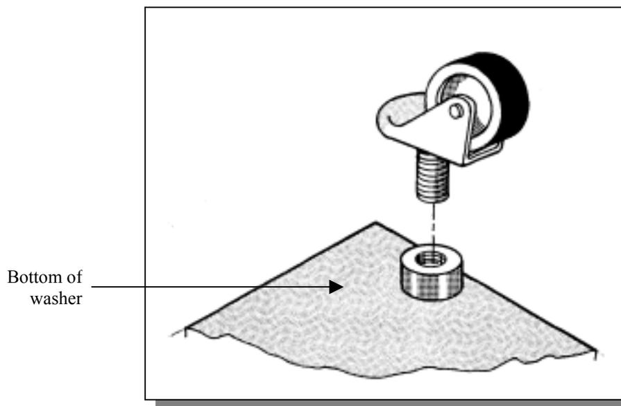
If you have the Undercounter or Freestanding model of the SteamScrubber or FlaskScrubber washer, refer to Figure 3-2 and follow the steps detailed below to install the leveling feet on your washer.
