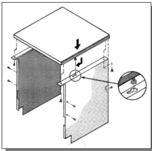
Remove four screws that attach the top to the sides. Then, slide the washer top toward the rear of the washer and lift to remove.
