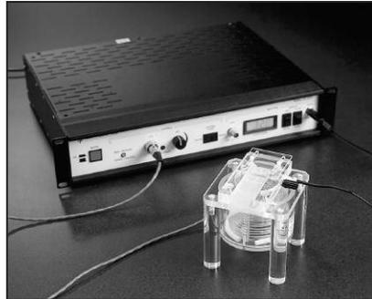
Figure 2. TC-202A Temperature Controller
