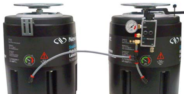
Figure 10— Detail of Valve Connections, Two Isolators
