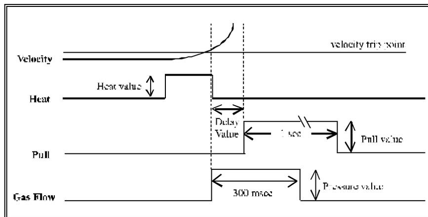
**Figure 11. Pull Cycle when DELAY > 0**
