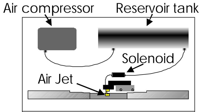
**Figure 7. P-97 Base Plate (Top view, cover removed)**
