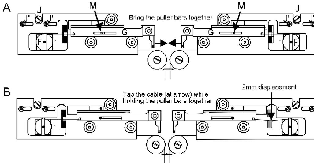
**Figure 26. Pulley Adjustment**
