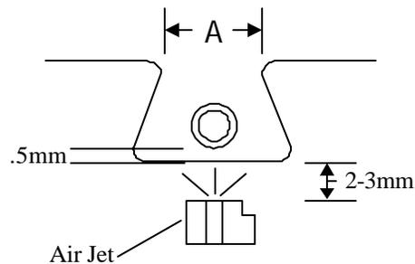
**Figure 21. End View of Trough Filament and Glass**
