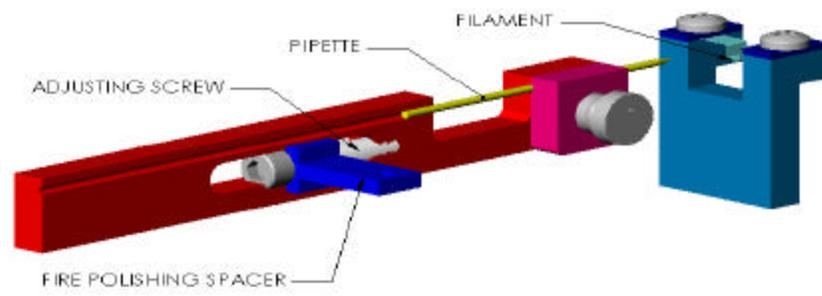
**Figure 20: Fire Polish Spacer in Puller Bar**
