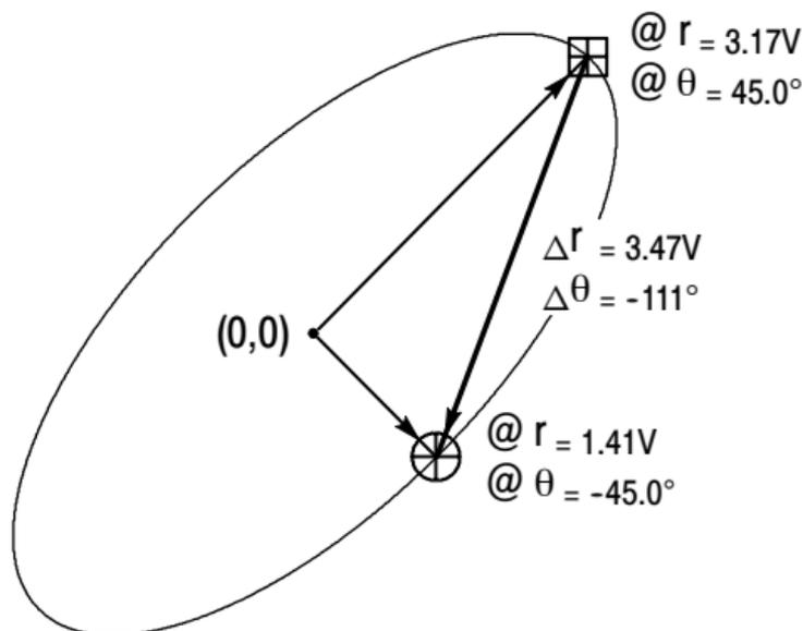
The following figure shows how the oscilloscope determines polar angle values.
