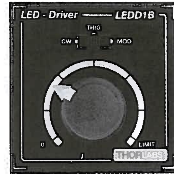
Operating Elements on the Top Panel
