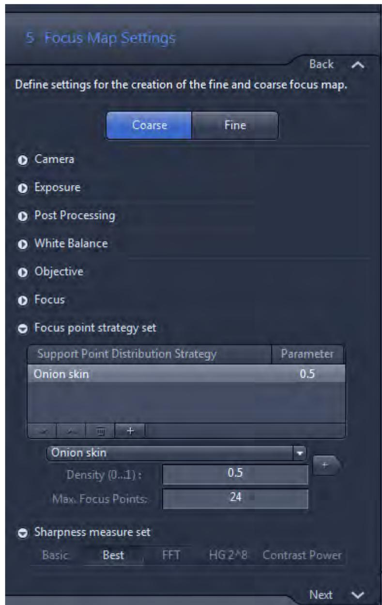
Appropriate focus map settings are important for ensuring good focus quality throughout the specimens. The focus map generation is done in two steps:
