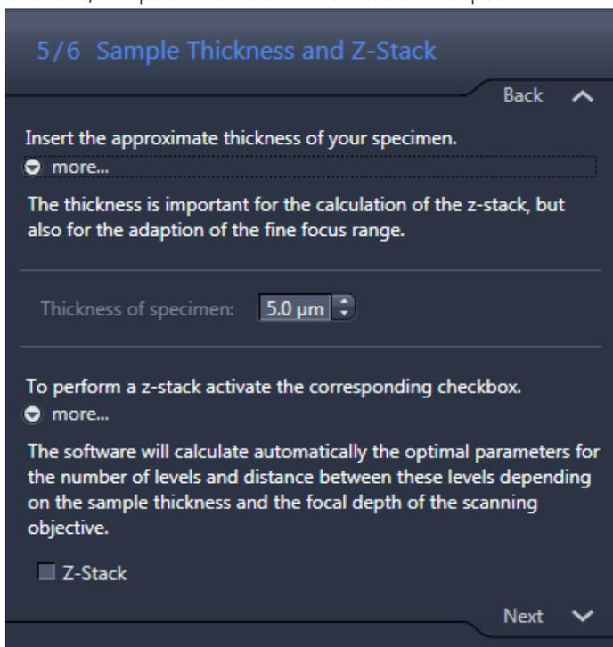
Based on this thickness, the software will calculate the number of focus levels and the distance of these levels based on the objective used. Finally, you can decide if the z-stack should be conserved or if an **EDF**
