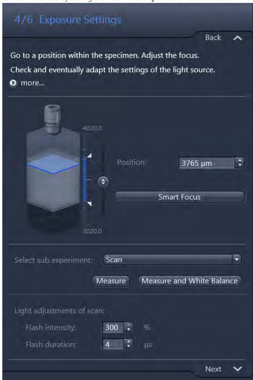
To adapt these settings (this is particularly necessary if the scanning objective has been changed) you should move the stage containing the specimen into
