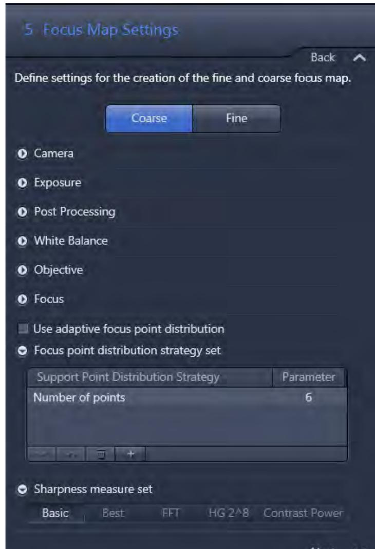
Appropriate focus map settings are important for ensuring good focus quality throughout the specimens. The focus map generation is done in two steps:
