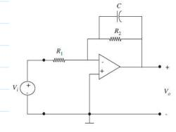
$$Q. \frac{V_{in}-V_{-}}{R_{1}} = \frac{V_{-}-V_{0}}{Z} \qquad \frac{1}{Z} = i\omega(+\frac{1}{R_{2}}) \implies Z = \frac{R_{z}}{1+i\omega R_{z}C}$$
