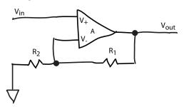
Only a fraction of the output voltage,  $V_-=rac{R_2}{R_1+R_2}V_{out}$  , is sensed. This forces the output voltage
