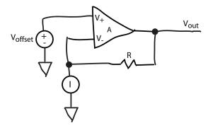
We have the node equation  $\frac{\left(V_{-}-V_{out}\right)}{R}=I$  as well as  $V_{out}=A\left(V_{+}-V_{-}\right)$ , so that  $V_{out}=\frac{A}{A+1}\left(V_{+}-IR\right)$  or  $V_{out}\xrightarrow{A\to\infty}V_{+}-IR$ . The input  $V_{+}$  is either grounded or set to an offset voltage  $V_{offset}$ .
