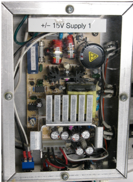
Figure 4 Custom electronics and software. (A) Power supply to drive the actuators in the scanning mirrors. (B) Screen shot of MPIScope 2.0 showing an example of a real-time image. (C) Power supply for the PMT. (D) I to V converter and pre-amplifier that sits between the PMT and the data acquisition board.
