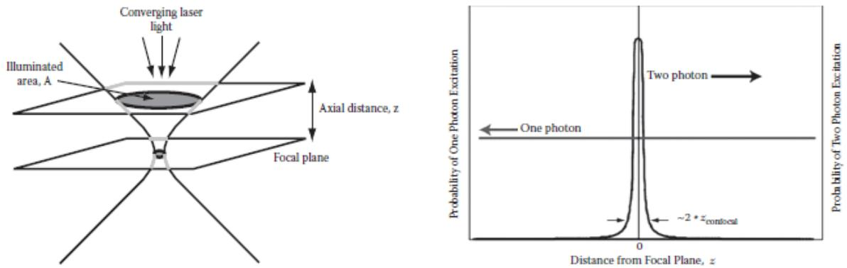
Figure 2: Due to the Quadratic Relationship between Intensity and Absorption, two photon has innately high z-resolution.
