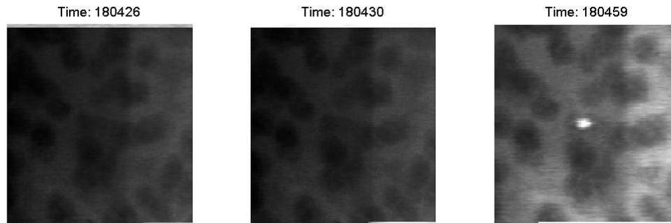
Figure 11: Three scans showing the time course of photobleaching. All images are taken at the same spot. Rastering was stopped between the second and third image. Titles are times in HHMMSS. Photobleaching occurs within 30 seconds upon exposure.
