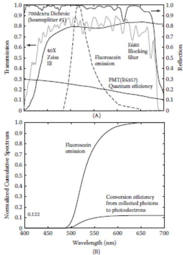
Figure 3: Photons emitted via fluorescence is much less than the reflected photon count from the incoming laser. Collection filters are necessary.
