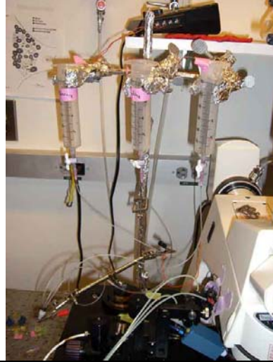
Fig 8 A perfusion setup to deliver leech saline followed by a 100uM solution of myomodulin.
