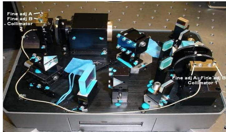
Fig 8. Picture of uncovered Clark MXR Modelocked laser [7]
