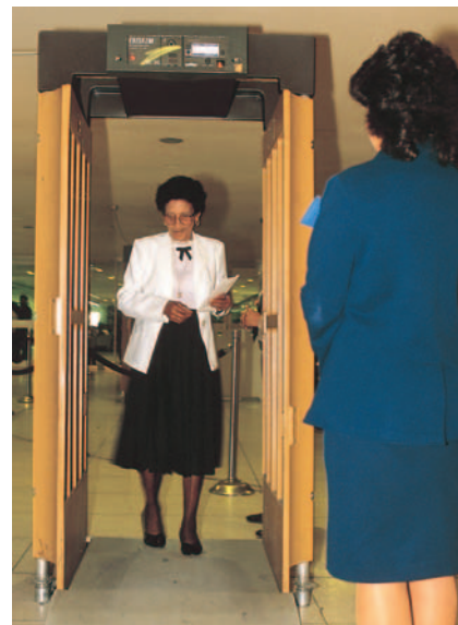
Figure 21.14 (Applying Physics 21.1) An airport metal detector.
