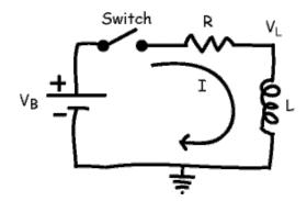
For the circuit above the initial current is zero and the switch is closed at time  $t = 0^{+}$ . We apply Kirchoff's Law, i.e., the sum of voltage drops around a loop is zero, and get:
