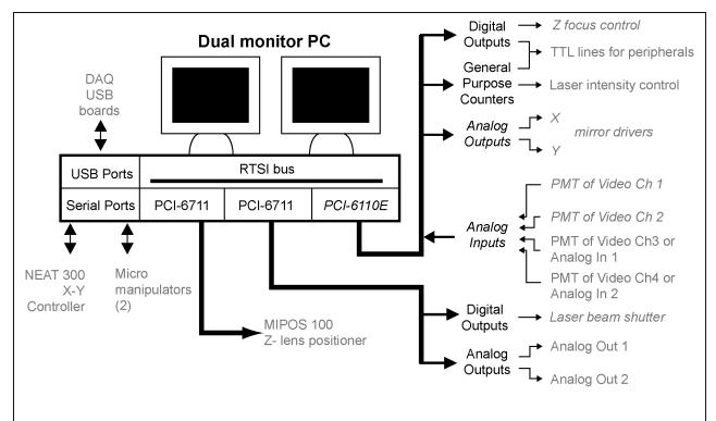
Fig. 1. Connection layout of MPScan in the original Kleinfeld configuration. Items in *italic* are mandatory. The PCI-6110E (or PCI-6115E) and the PCI-6711(s) have their RTSI buses tied together.
