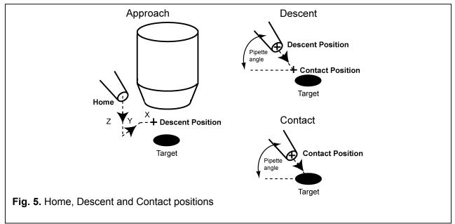
At this stage, the user can register the Home position of the pipette. To register the position of the target cell, the user will move the cell at the center of the crosshairs using the microscope translation controls and click on the Register Target button.
