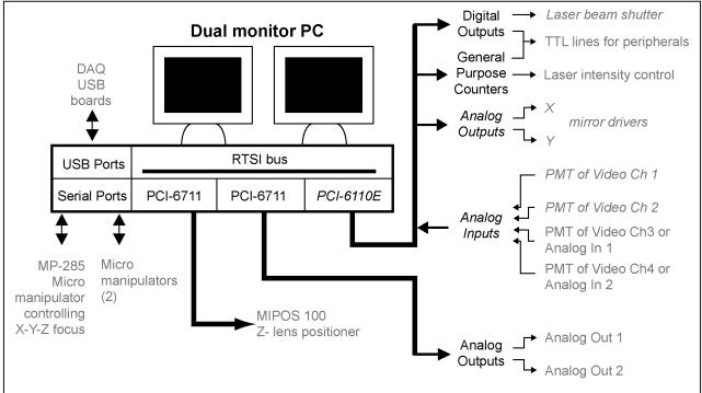
Fig. 2. Connection layout of MPScan in the Denk or Svoboda scopes. Items in *italic* are mandatory. The PCI-6110E (or PCI-6115E) and the PCI-6711(s) have their RTSI buses tied together.
