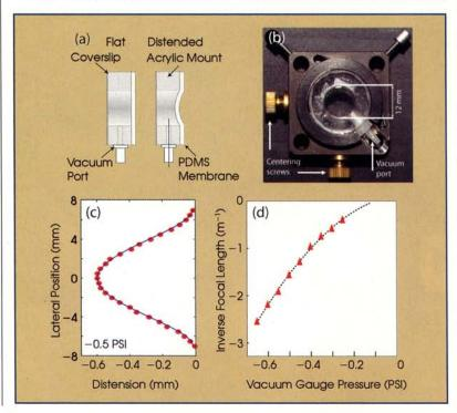
Israel. The investigators designed and demonstrated a deformable membrane that improves the axial resolution of twophoton microscopes twofold.
