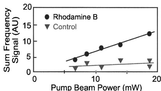
FIG. 1. A single-trial TPA measurement on rhodamine B (8.3 mM in methanol) at  $\lambda_0=880$  nm shows the linearity of the sum-frequency signal with the pump beam power. Control data are collected with the rhodamine sample placed in the beam path but outside of the focal region.
