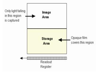
Figure 7: Frame Transfer CCD
