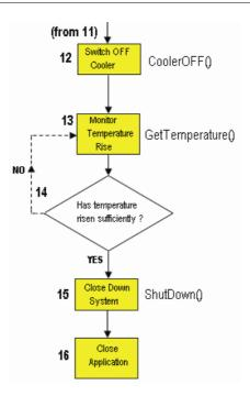
**12.** When the user has completely finished acquiring data the shutdown procedure is started. The cooler is switched off. It is important to control both the heating and cooling rates of the CCD sensor otherwise the temperature gradients may damage the sensor. Thus it is **highly recommended** that the user uses the correct exiting procedure rather than, for example, simply switching off the computer.
