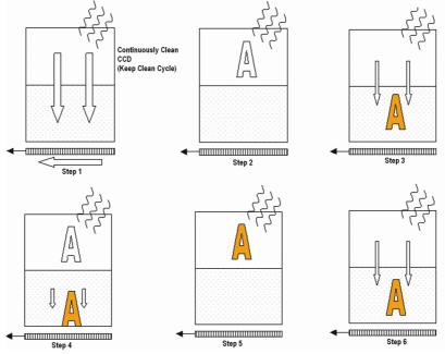
Figure 8: Capture sequence for a Frame Transfer CCD
