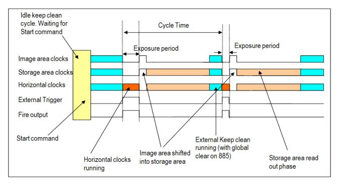
External Exposure Trigger in Non-Frame Transfer mode
