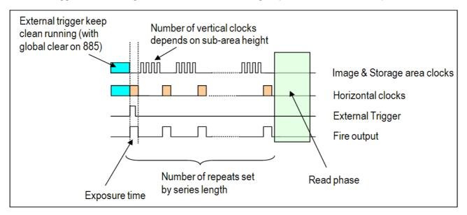
External Start trigger in Fast Kinetics mode
