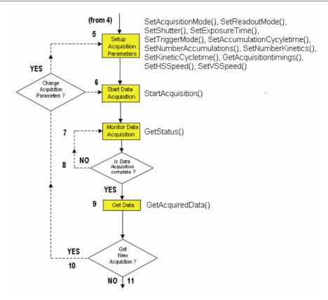
**5.** The acquisition parameters are programmed to match the specifications of the user, e.g. acquisition mode (single scan etc.), readout mode (full vertical binning etc.) and the trigger mode (Internal etc.).
