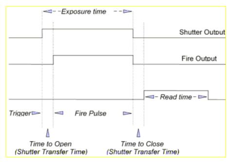
Internal Trigger Mode is ideal for situations where you are using 'continuous wave' (CW) light sources (an ordinary room light for instance) and incoming data, for the purposes of your observation, are steady and unbroken: thus you can begin acquisitions 'at will'.
