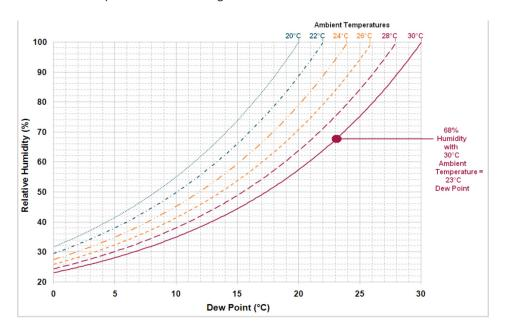
Figure 26:Calculation of dew point from ambient temperature and relative humidity
