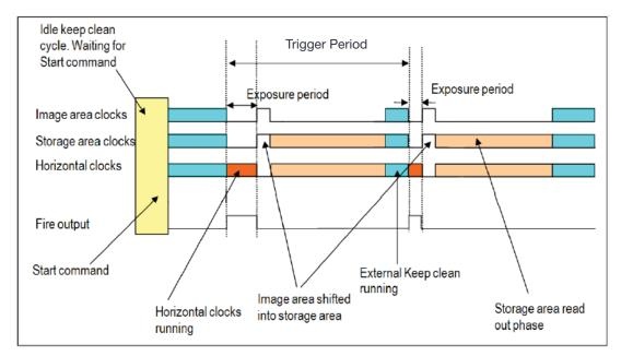
Figure 19: Internal Trigger in Non-Frame Transfer Mode.
