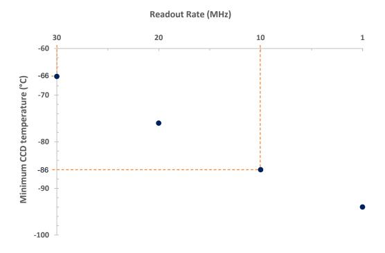
Figure 8: Minimum achievable temperature at each of the horizontal readout speeds for full frame readout and keeping all other parameters the same (Air cooled 20 °C ambient).
