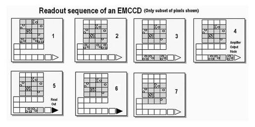
Figure 28: Readout sequence of an EMCCD
