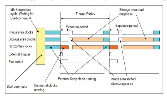
Figure 20: External Trigger in Non-Frame Transfer Mode
