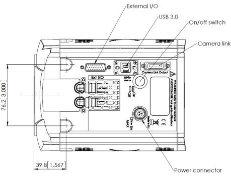
Figure 3: Power and Signal Connections of the Ixon Ultra 888
