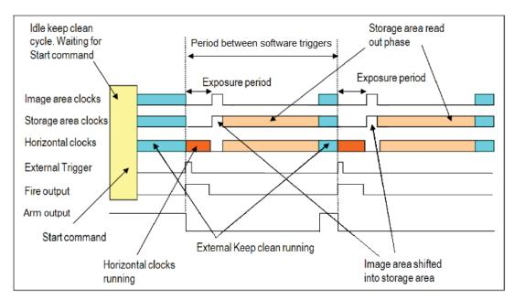
Figure 22: Software Triggering in Non-Frame transfer Mode
