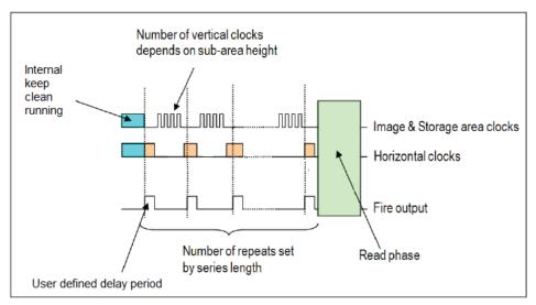
Figure 23: Internal Triggering in Fast kinetics Mode.
