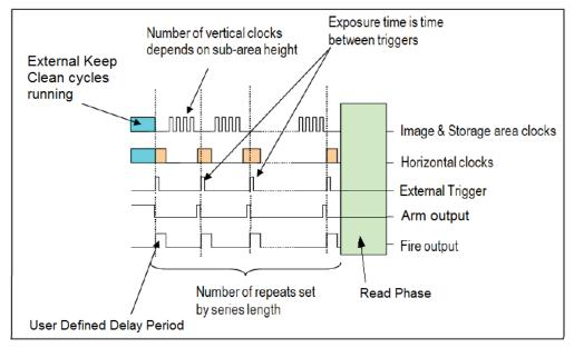
Figure 24: External Triggering in Fast Kinetics Mode
