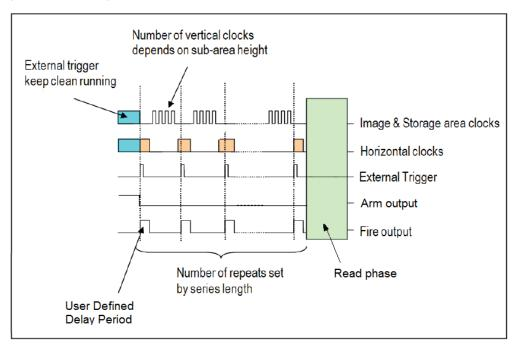
Figure 25: External Start Trigger in Fast Kinetics mode
