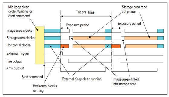
Figure 16: External Trigger in Frame transfer Mode
