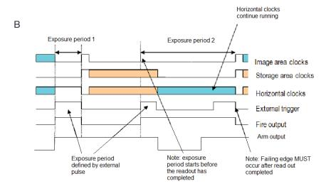
Figure 18: External Exposure Trigger in Frame Transfer Mode
