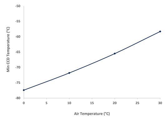
Figure 7: Minimum CCD temperature at varying air temperature.
