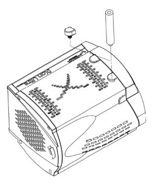
Figure 10: Attaching the Mounting Posts
