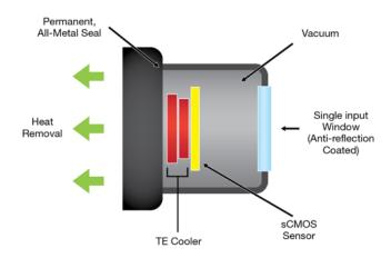
Figure 27:Ultravac™ metal hermetic vacuum sealing
