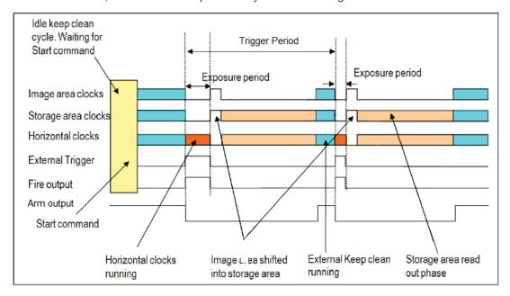
Figure 21: External Exposure (NFT) Triggering
