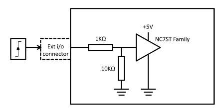
Figure 5: External Trigger
