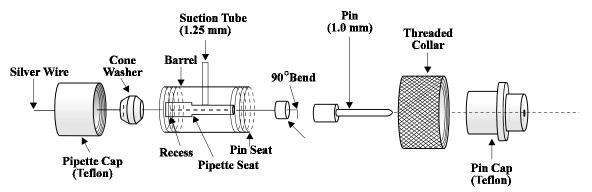
Figure 15. Exploded view of the holder
