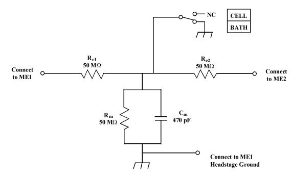
Figure 10. CLAMP-1U model cell
