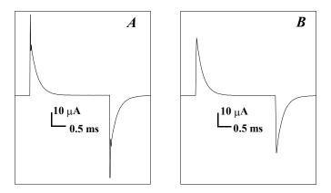
Figure 8. Tuning the TEVC with the MCO-1U model cell
