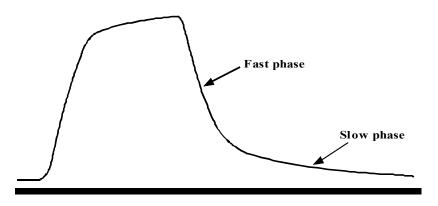
Figure 9. Two-phase microelectrode decay
