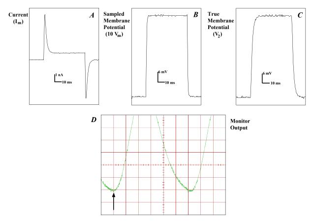
Figure 6. Incorrectly set up dSEVC (i.e., "False" clamp) in a cell model
