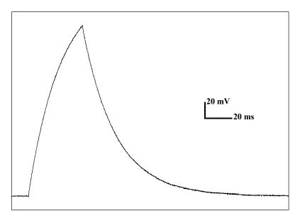
Figure 2. Correctly adjusted bridge and capacitance neutralization controls using the CLAMP-1U model cell
