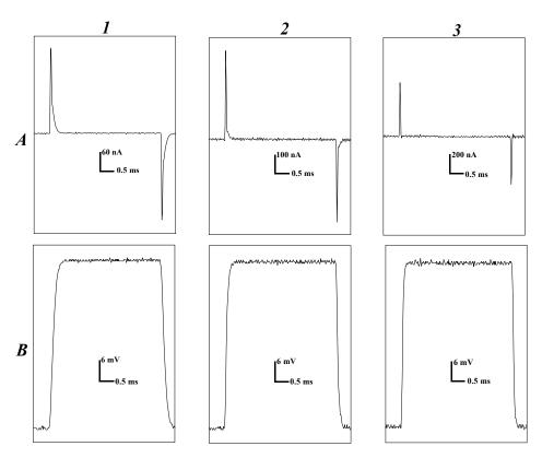
Figure 7. Tuning the TEVC with the CLAMP-1U model cell
