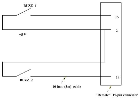
Figure 18. External switch wiring diagram
