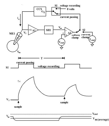
Figure 23. dSEVC block diagram and timing waveforms
