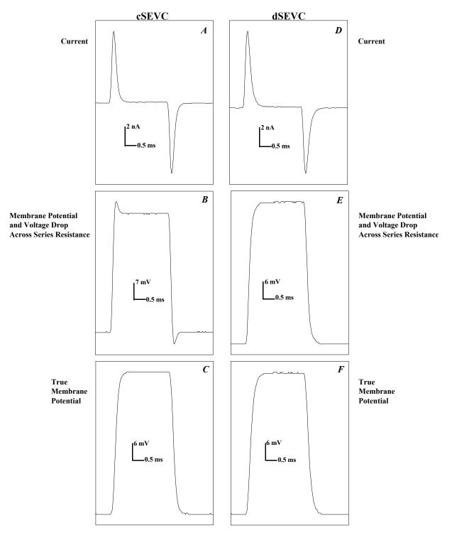
Figure 24. Comparison of current and potential during dSEVC and cSEVC using the MCW-1U model cell
