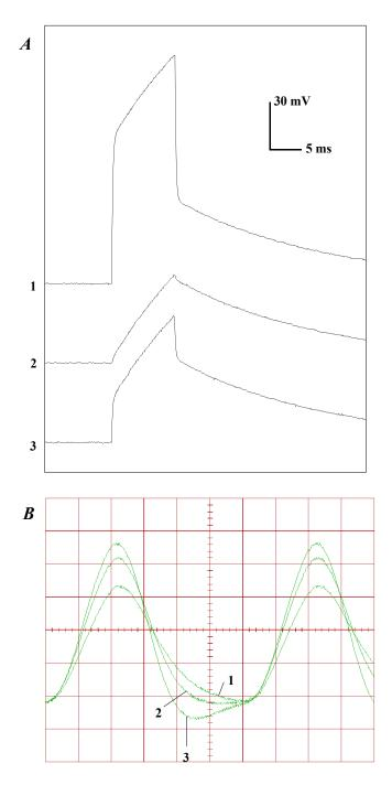
Figure 4. How to set the capacitance neutralization during DCC mode
