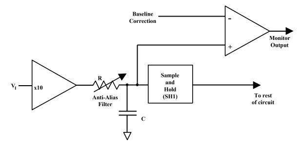
Figure 17. Anti-alias filter and monitor circuit
