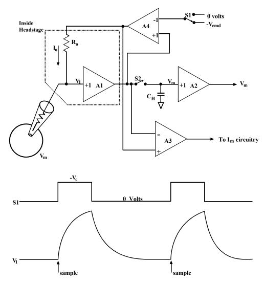
Figure 22. DCC Mode block diagram and timing diagram
