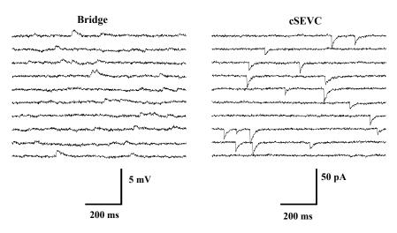
Figure 21. Recordings from brain slices in bridge mode and cSEVC mode
