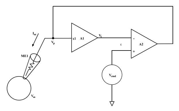
Figure 20. Simplified schematic of cSEVC
