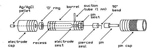
The various parts of the holders are shown in the exploded view:
