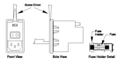
Note: A non-operator-replaceable fuse exists inside of the equipment. This fuse is rated T 40mA 250V, 5 x 20mm.
