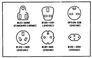
Figure 2-2. Power Cord Plug Configurations
