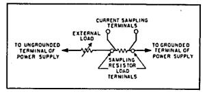
Figure 5-2. Current Sampling Resistor Connections
