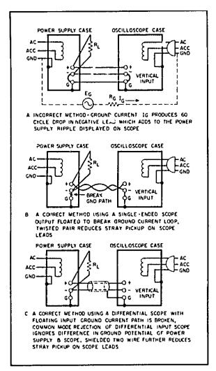
Figure 5-4. Ripple and Noise, Test Setup
