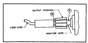
Figure 5-1. Front Panel Terminal Connections
