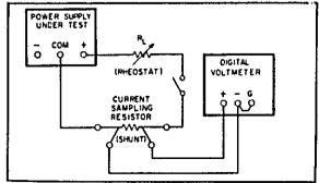
Figure 5-3. Output Current, Test Setup
