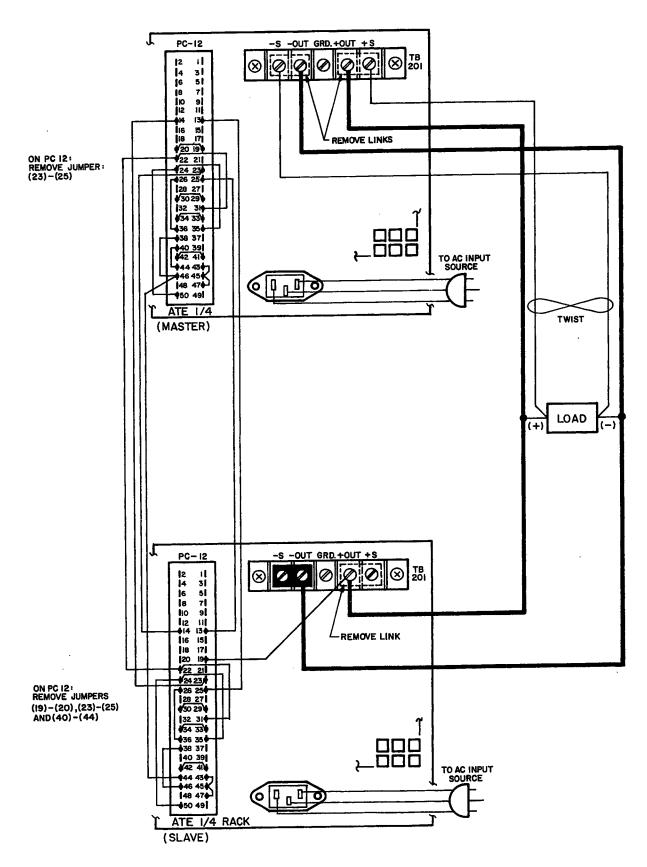
FIG. 3-26 MASTER/SLAVE PARALLEL CONNECTIONS
