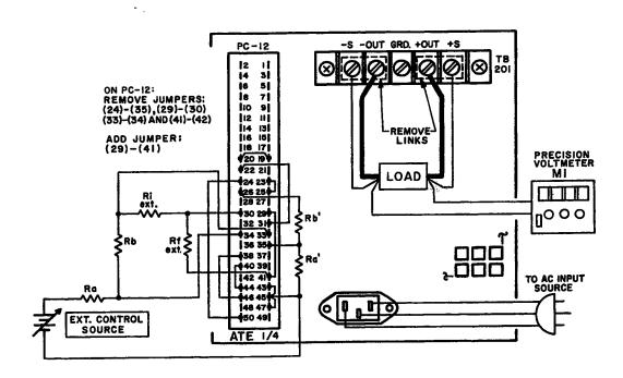
FIG. 3-30 CONNECTIONS FOR PROGRAMMING WITH REFERENCE TO THE NEGATIVE POWER SUPPLY OUTPUT.
