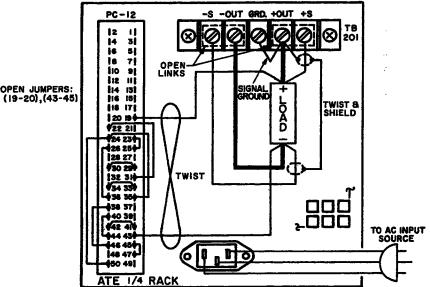
FIG. 3-5 LOAD CONNECTION, METHOD III.
