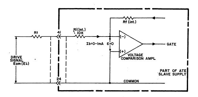
FIG. 3-21 DEVELOPING THE DRIVE FOR THE MASTER/SLAVE SERIES CONNECTION, ATE POWER SUPPLIES WITH RATED OUTPUT VOLTAGE > 6V.
