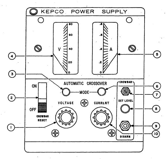
FIG. 2-2 CONTROLS AND TERMINATIONS, ATE 1/4 RACK GROUP, FRONT.
