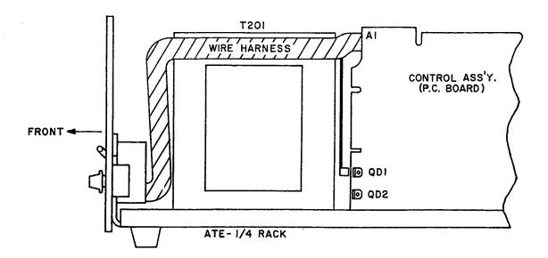
FIG. 2-5 LOCATION OF INTERNAL SIGNAL GROUND, SIGNAL GROUND NETWORK SHOWN CONNECTED VIA QD-1. TO REMOVE SIGNAL GROUND, PLACE WIRE LUG ONTO QD-2.
