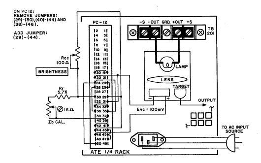
FIG. 3-18 CONNECTIONS FOR ILLUMINATION CONTROL, USING THE EXT. CURRENT COMPARISON AMPL.
