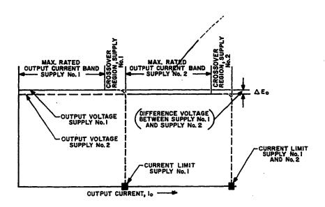
FIG. 3-24 "AUTOMATIC" PARALLEL OPERATION (TWO SUPPLIES).
