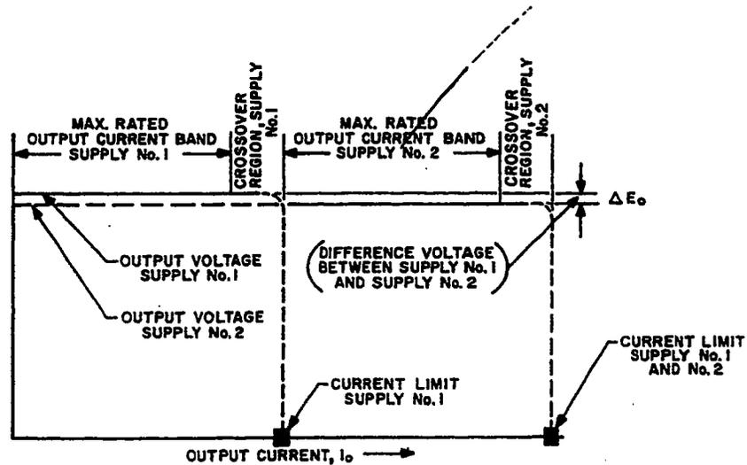
FIG. 3-24 "AUTOMATIC" PARALLEL OPERATION (TWO SUPPLIES).
