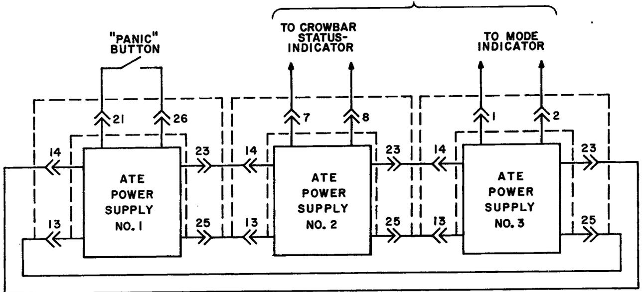
FIG. 3-19 MULTIPLE POWER SUPPLY FAULT DETECTION LOOP
