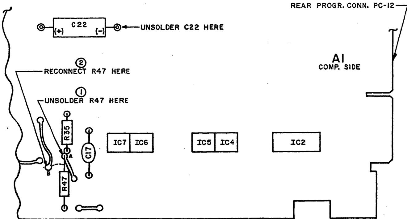
FIG. 3-27 LOCATION OF OVERVOLTAGE SENSING LEAD DISCONNECT.
