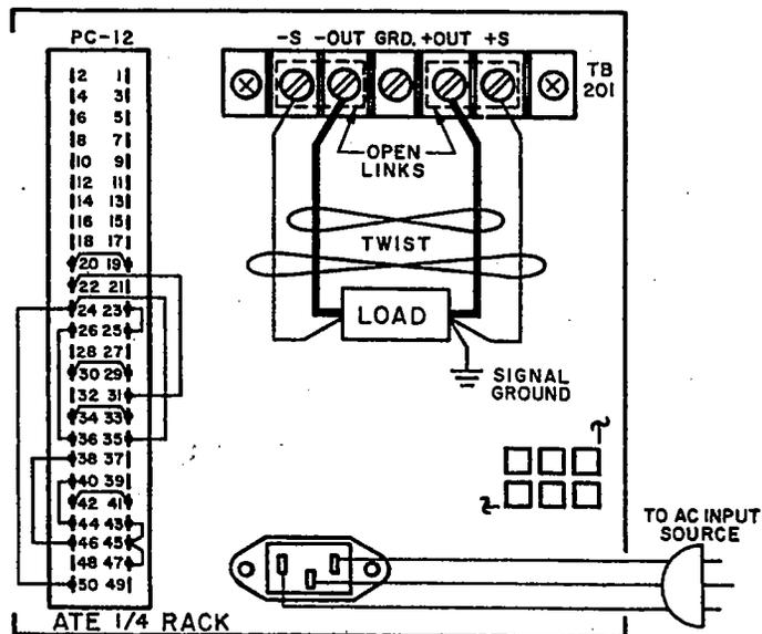
3-23 This method of load interconnection is suitable for loads which do not require rapid changes in voltage or current or for programming with gradually changing waveforms (sine wave, triangular wave shapes, etc.). See par. 3-24 for load connections suitable for rapid (step) changes in the load or in programming.
