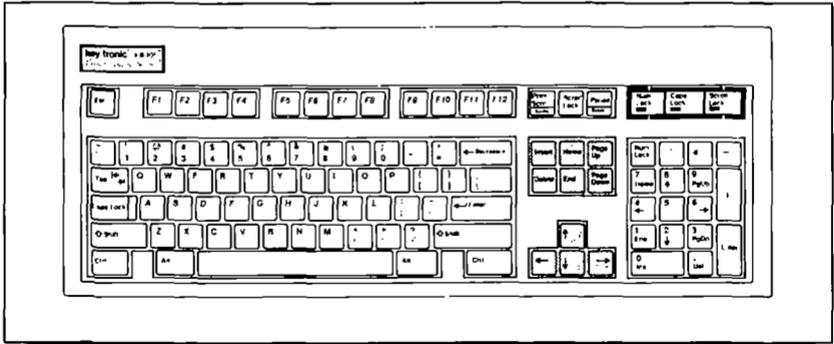
The KB 101 keyboard features a separate cursor control keypad. This keypad is active during all modes of keyboard operation and is especially convenient when the numeric keypad is in numbers mode (Num Lock LED is ON).
