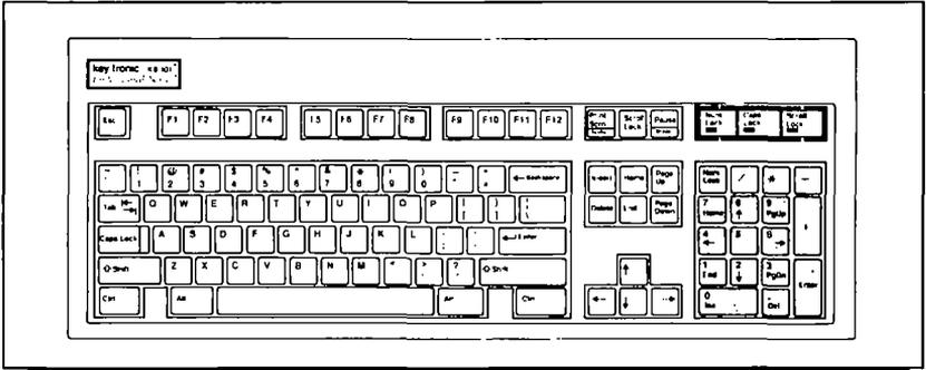
The numeric keypad provides a quick, easy way to enter numeric values while still having a separate cursor control keypad for cursor positioning and edit functions. All four common math function signs: /, \*, - and +, are on the numeric keypad.
