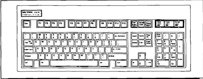
The KB 101 has twelve multi-purpose *function keys*, F1 through F12, located across the top of the keyboard for easy access. The function of each key is defined by the application program you are using.
