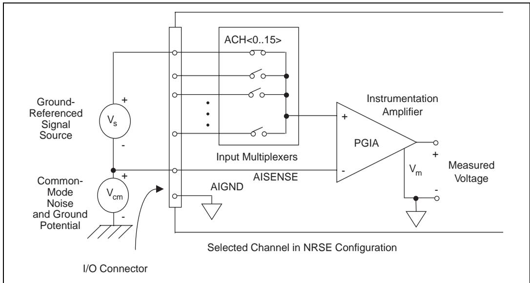
**Figure 4-9.** Single-Ended Input Connections for Ground-Referenced Signal
