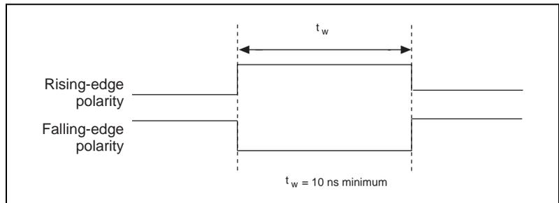
**Figure 4-35.** GPCTR1\_GATE Signal Timing in Edge-Detection Mode
