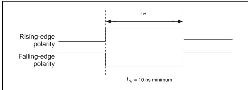
**Figure 4-32.** GPCTR0\_GATE Signal Timing in Edge-Detection Mode
