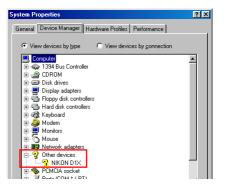
If "Nikon 1394 Protocol Device" is not listed in the Device Manager and "NIKON DIX(DI/DIH)" is not listed under Other Devices, re-start your computer and return to Step 1.
