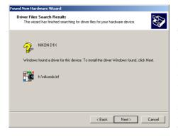
If the message, "Windows was unable to find a suitable driver for this device," is displayed, this may indicate that the Nikon View 4 CD was not correctly inserted in the CD-ROM drive or that the correct search location was not specified. Click **Back** to return to the dialog shown in Step 3, where you can confirm that the correct location has been specified.
