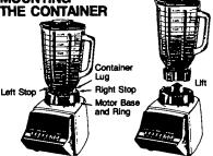
To operate blender, place assembled container in base ring with container lug against flat side of right motor base stop. If container lug does not rest against flat side of right stop, remove container assembly and place against flat side of left stop. Seat container firmly and operate.
