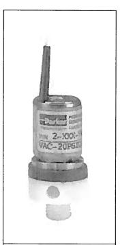
All Series 2 valves are cycled 50,000 times prior to shipment after which they are tested 100% for all electrical and flow characteristics including actuation, response time, and leakage under both pressure and vacuum. After this rigorous testing, they are put through one additional leak check on a Mass-Spectrometer and tested for leak rates less than 1x10<sup>-6</sup> ATM-cc/sec Helium.
