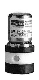
The Series 1's small internal volume combined with a fast response time—8ms—enables users to get fast readings and analysis. Washout is rapid. The Series 1's require no pressure to operate and the absence of sliding surfaces in the fluid stream ensures operation without particle generation.
