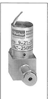
The Series 9 is designed for high speed (5 ms or less opening response time) high flow (up to .116" orifice size) and high temperature applications (up to 200° C). This highly reliable compact valve is perfect for applications with the most critical needs. All valves are tested on helium leak detector mass spectrometers for leak rates less than 1 x 10-7 cc.
