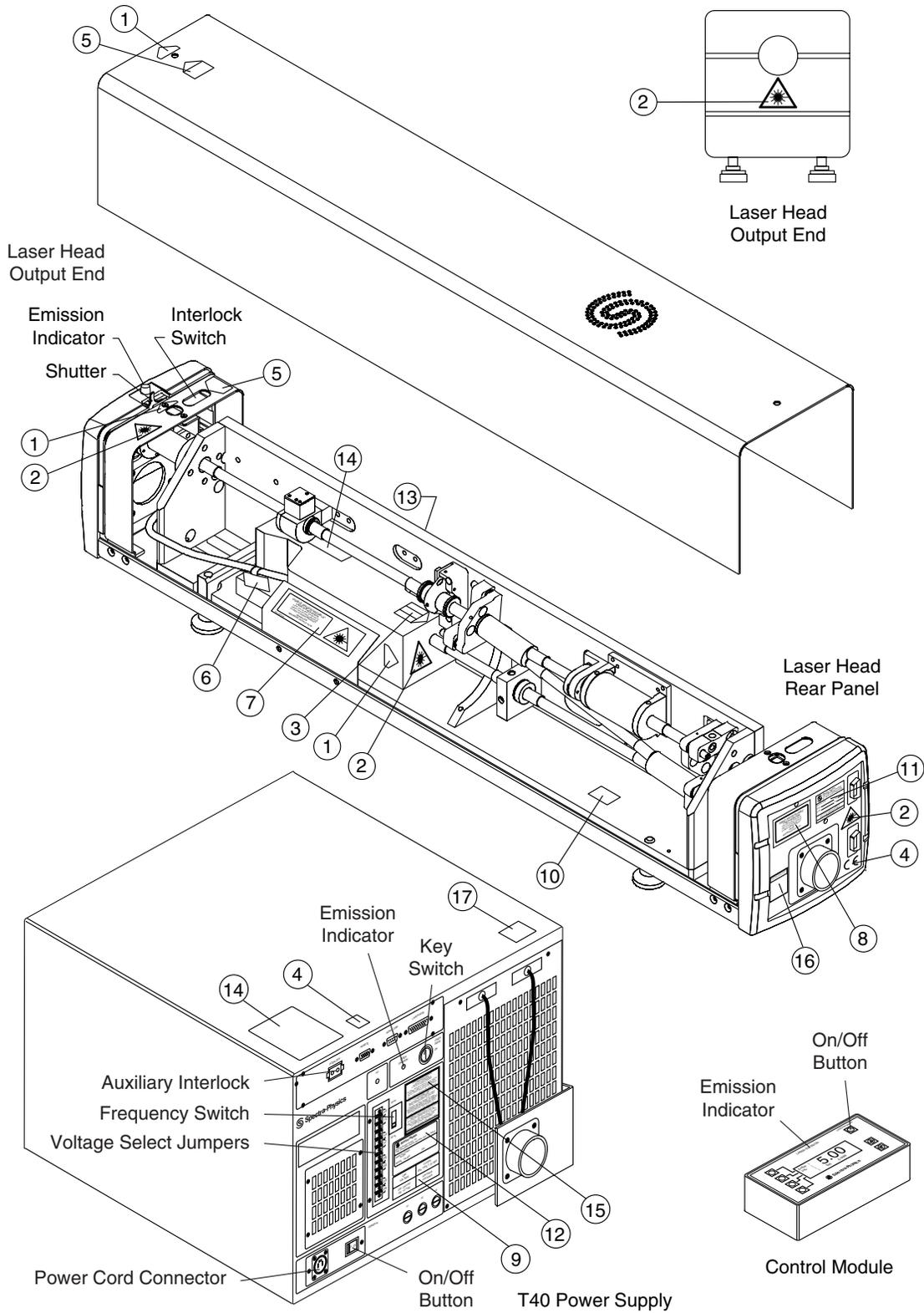
Figure 2-5: CE/CDRH Radiation Control Drawing
