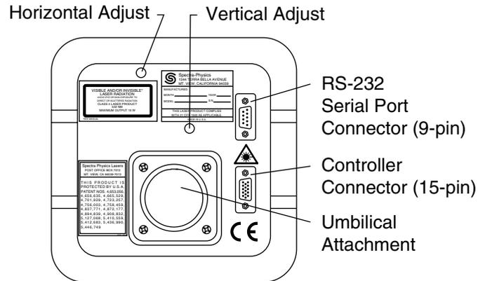
**Figure 4-2: The *Millennia V* Laser Head Rear Panel**
