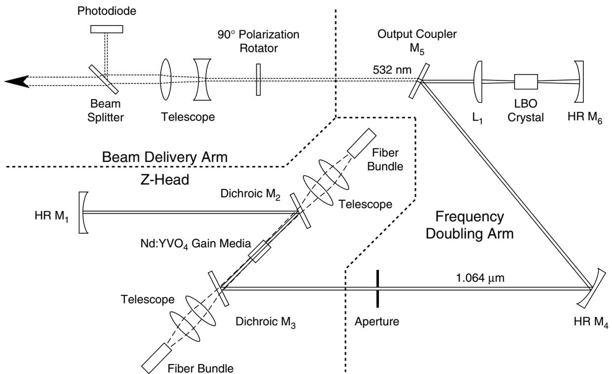
**Figure 3-10: Schematic of the *Millennia V* Laser Head**
