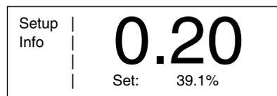
To change the power or current setpoint, either press one of the preset power setpoint keys, P1 or P2, to move directly to a preset power (set in the Setup menu), or use the up/down buttons to set a new value. Note that when the buttons are held down, the setpoint numerical update pauses from time to time. This is normal. To change from power to current mode, or vice versa, use the Setup menu.
