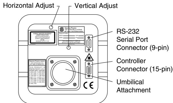
**Figure 5-1: The *Millennia V* Laser Head Rear Panel**
