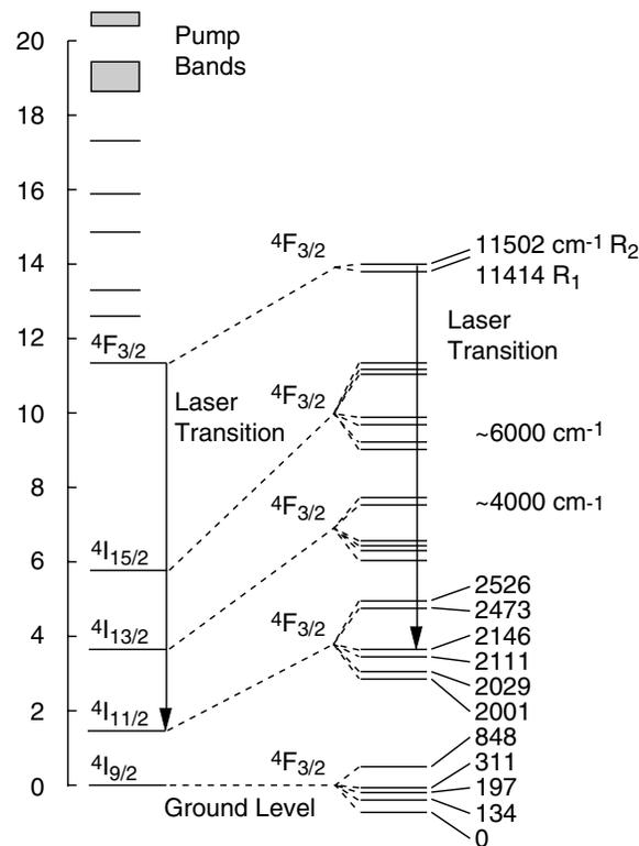
**Figure 3-4: Energy Level Scheme for the  $Nd^{3+}$  Ion.**
