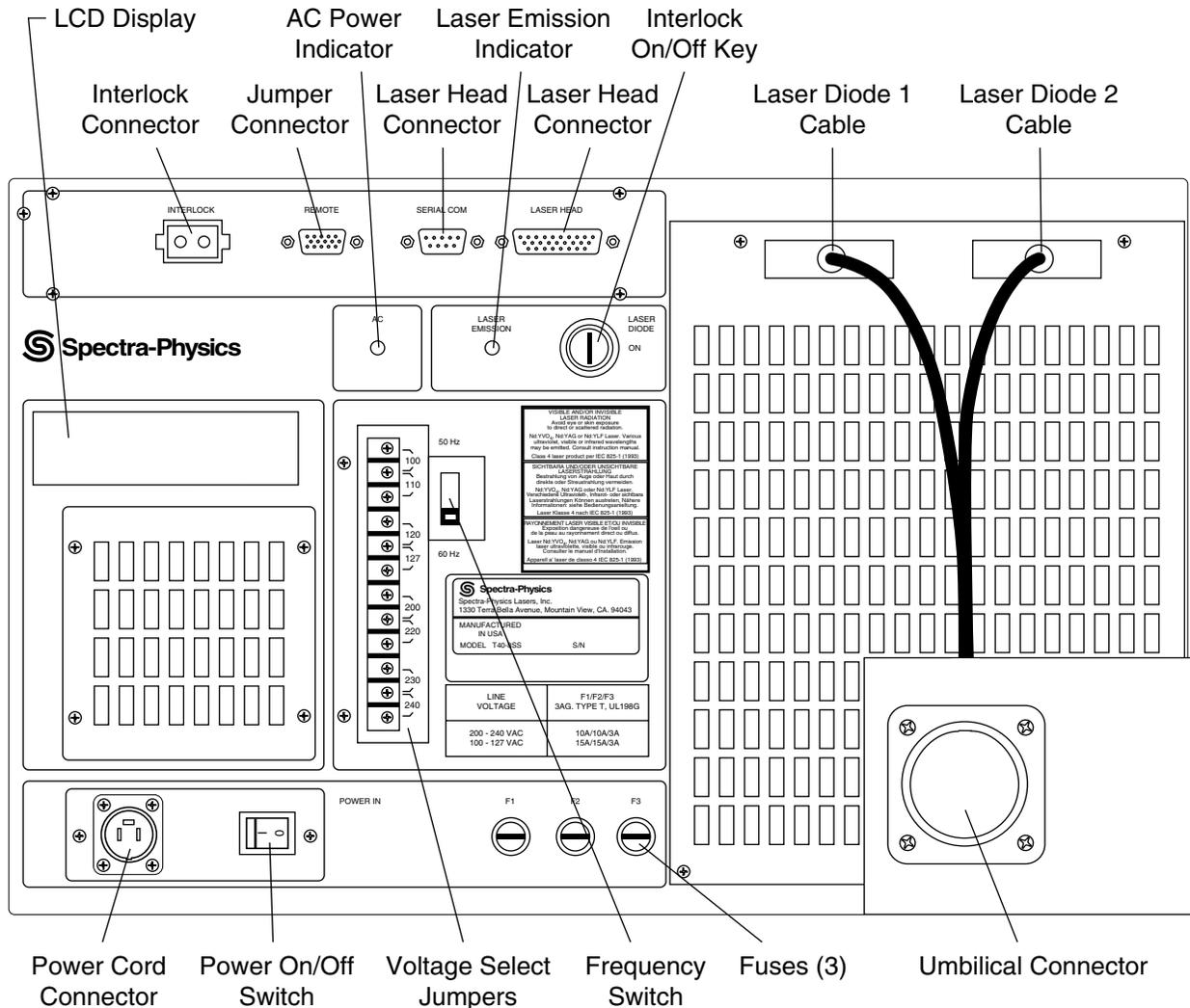
Figure 4-4: The Model T40 Power Supply Control Panel
