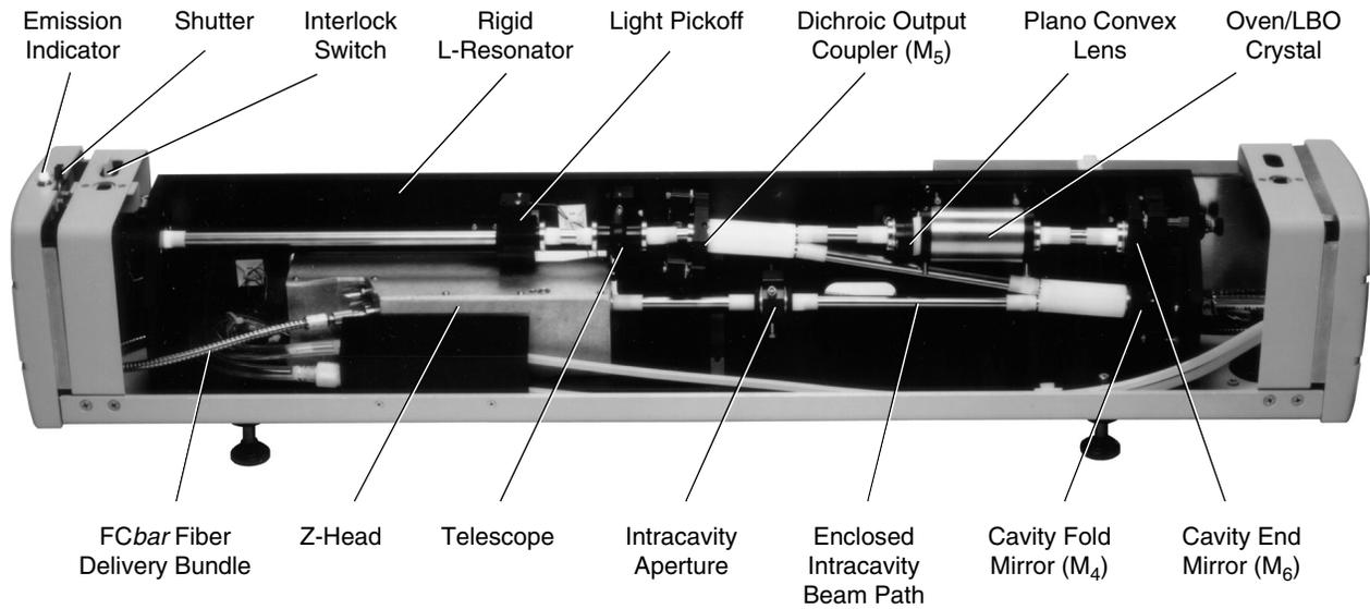
**Figure 3-9: The *Millennia V* Laser Head**
