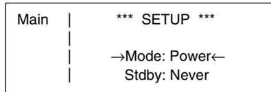
Use the two lower left buttons to scroll the menu up and down; the “selected” item is the one between the horizontal arrows (“Mode: Power” in the example screen above). The value for the “selected” item is changed by using the up/down buttons to the right of the screen. The selections and/or changes are activated upon return to the Main menu. Selections include:
