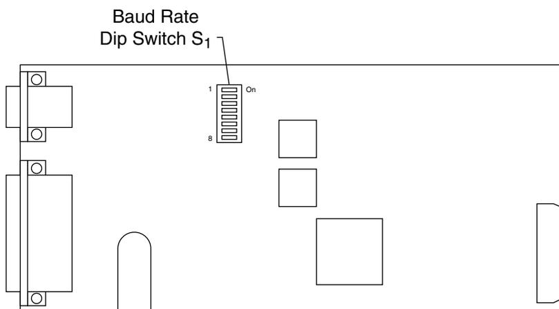
**Figure 6-4: Laser head pc board showing the location of baud rate dip switch S<sub>1</sub>.**
