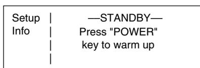
1. Press the LASER POWER button to begin the short warm-up cycle. The following prompt is displayed for about 2 minutes while the diode temperature stabilizes:
