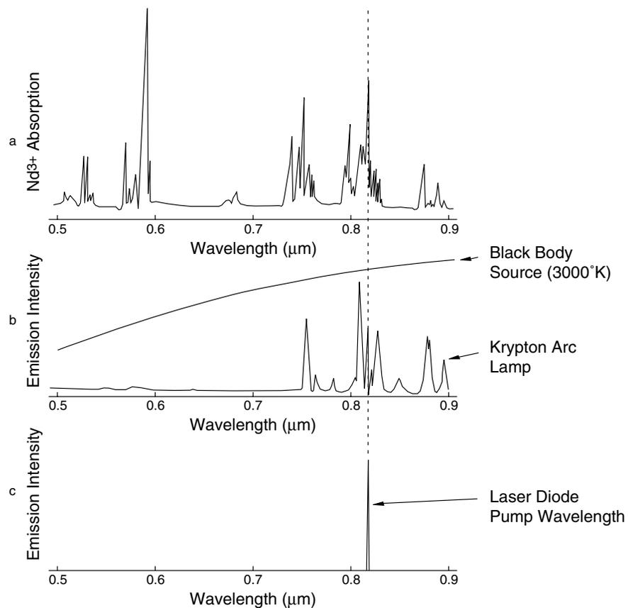
**Figure 3-5: Nd<sup>3+</sup> absorption spectra compared to emission spectra of a Black Body Source (a), Krypton Arc Lamp (b) and a Laser Pump Diode (c).**
