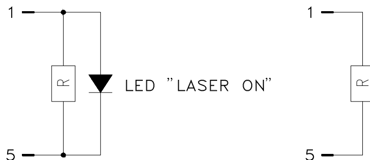
Figure 4 Connecting the interlock with and without monitoring LED
