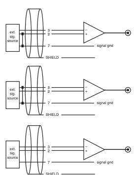
**Figure 2** BP 1 connected to an external signal source. Upper, single ended, inverting. Middle, single ended, non-inverting. Lower, differential.
