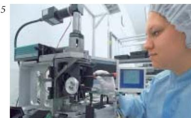
In the zoom body adjusting device, the precise procedures of all moveable optical elements are programmed. To do this, approximately 7,000 reference points are analyzed by computer. In doing so, each stereomicroscope receives its own completely individual zoom control curve.
