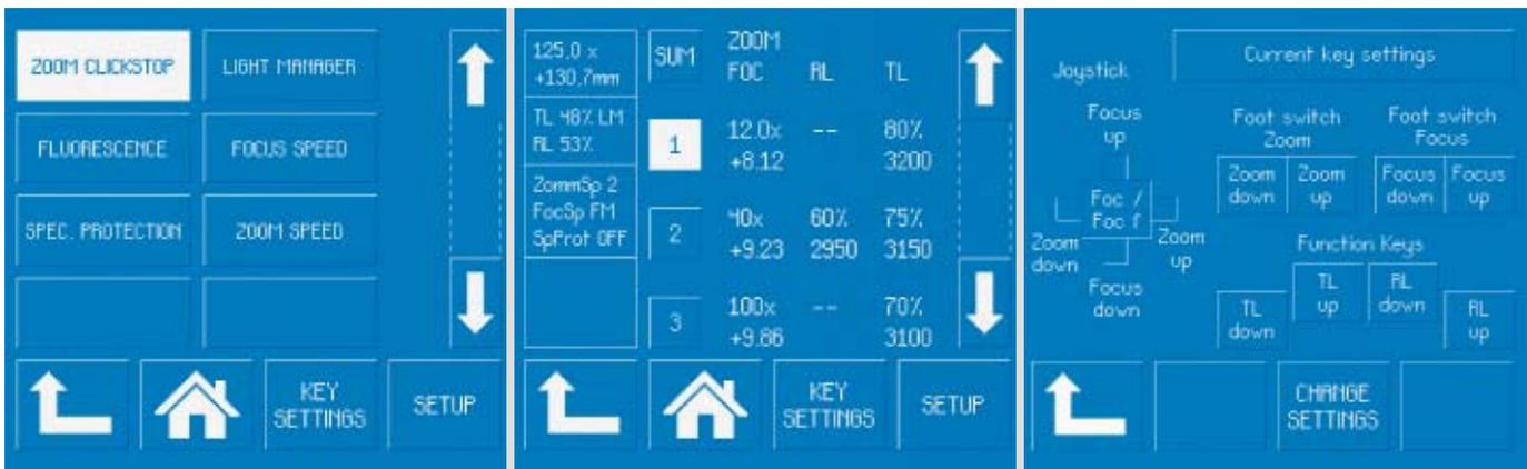
In the **FUNCTION** menu it is possible, for example, to set ClickStops, activate electronic specimen protection, select speeds for zooming and focusing and activate the light or focus manager.
