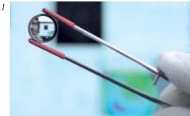
Before assembly begins, each lens is exactly calibrated against a reference "null lens set" and the values are saved in a data pool. This feeds the database used by a computer to select optimally matched lenses for the zoom system. By doing this, an optimally coordinated lens family is developed for every stereomicroscope.
