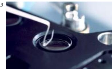
... the moveable micro clapper on the computer controlled glue leveling machine automatically adjusts the final fine alignment.
