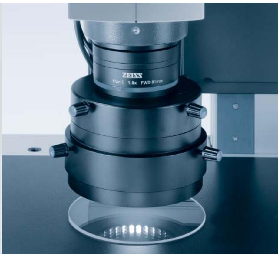
In order to combine brightfield and darkfield in reflected-light, the **VisiLED ring light S 40-10 DF** is mounted onto the brightfield ring light using a special adapter.
