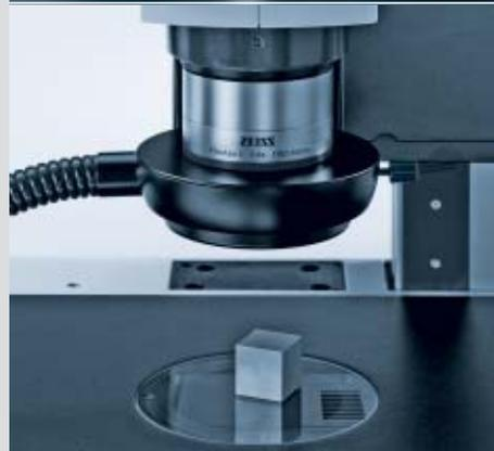
The better a specimen is illuminated, the more details it reveals to the observer. For example, fiber optic illumination components optimized for different applications generate very specific lighting effects on the surface of the specimen. The range extends from simple spot illuminators and ring lights through to specifically shaped glass fiber bundle geometries.
