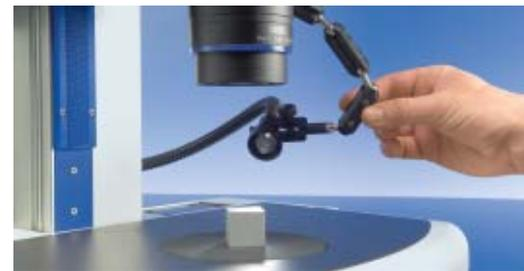
*Extremely precise alignment of the illuminator is a must in order to achieve good 3D contrast in oblique reflected-light. Special clamps, illuminator carriers and articulated arms are available to ensure that the fixing is exact. Focusing attachments help to concentrate the light on the object field.*
