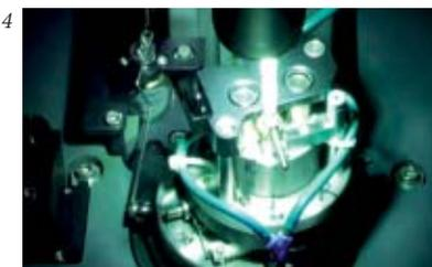
The lens which has been positioned carefully is then fixed immediately. The machine lays highly calibrated, uninterrupted glue beads through a strong 0.5 mm cannula and hardens it using UV light.
