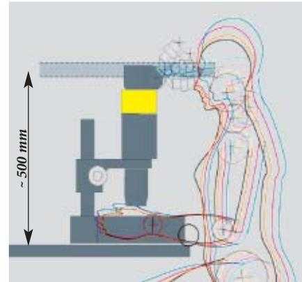
According to the results of an international study, a viewing height of approx. 500 mm with a viewing angle of around 20 degrees is best for avoiding tension and neck pain when using a microscope.
