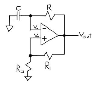
The time-varying voltage at  $V_+$  serves as a target level that is a fraction  $R_2/(R_1+R_2)$  of the output voltage  $V_{out}$ . The time-varying voltage at  $V_-$  heads toward this value and when it exceeds the value, the output of the amplifier changes sign, thus the target changes sign, and the voltage at  $V_-$  heads toward this new value.
