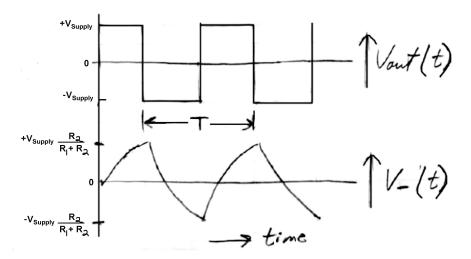
At t = T/2 the value of V\_(t) will reach the threshold level
