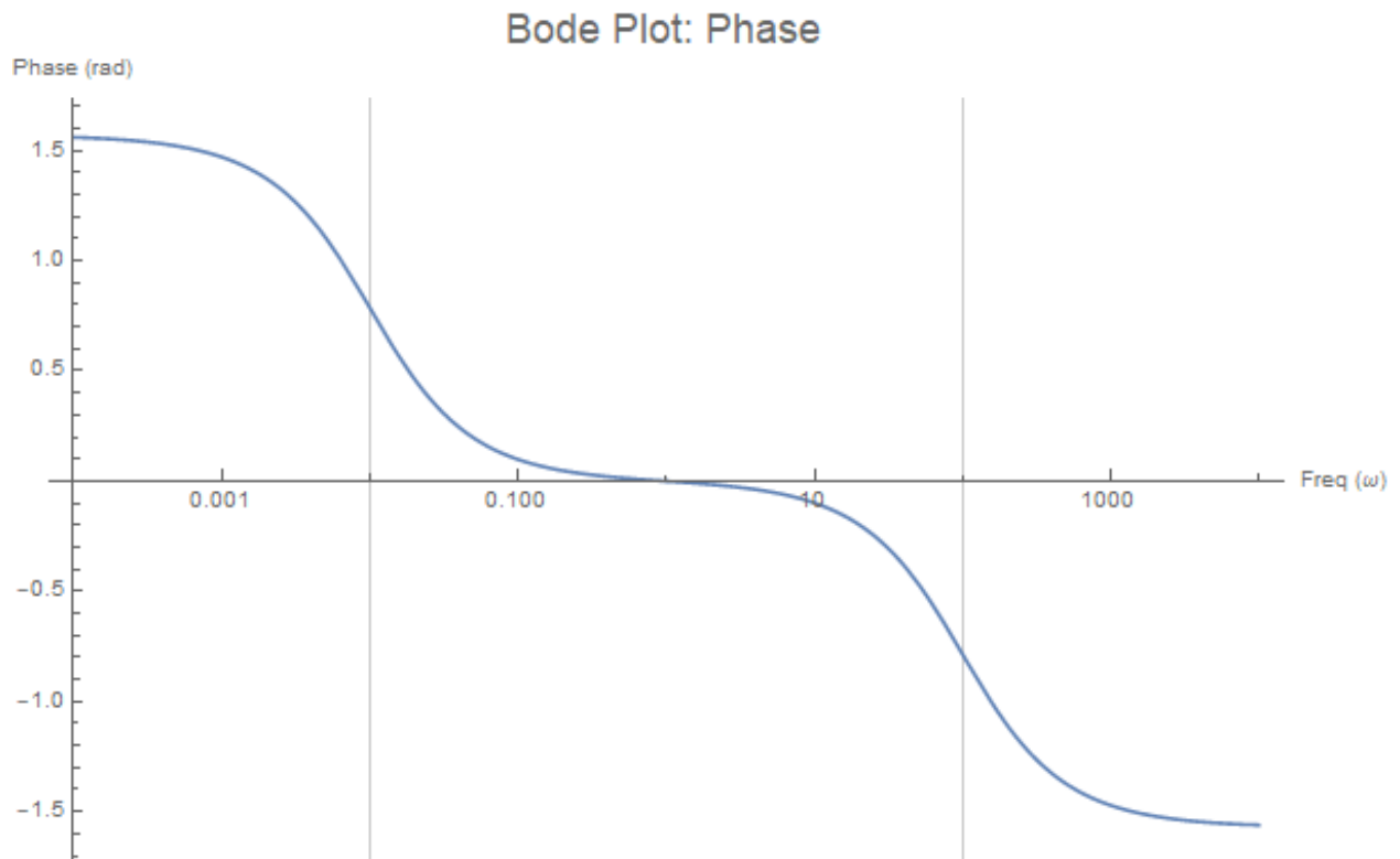
Figure 6: Bode plot. Values chosen: R_f = 10 \text{ k}\Omega and C_f = 1 \text{ }\mu\text{F} , R_{in} = 1 \text{ M}\Omega and C_{in} = 100 \text{ }\mu\text{F} .
