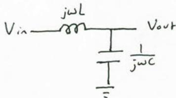
$$\frac{V_{out}}{V_{in}} = \frac{\frac{1}{j\omega C}}{j\omega L + \frac{1}{j\omega C}} = \frac{1}{1 - \omega^2 LC}$$
