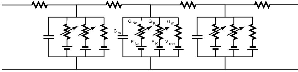
Figure 6.12: ELECTRICAL CIRCUIT OF THE SQUID GIANT AXON
