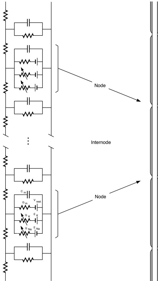
Figure 6.15: ELECTRICAL CIRCUIT FOR A MYELINATED AXON
