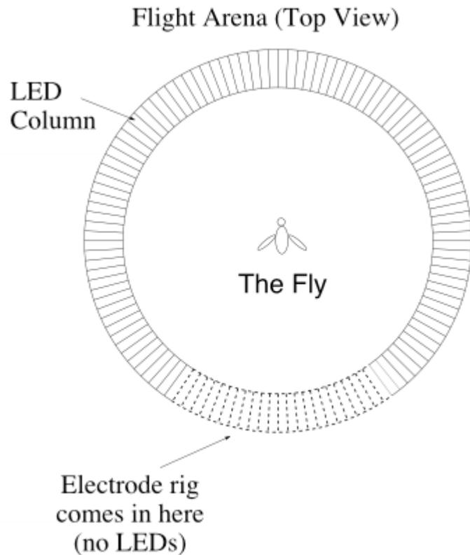
The H1 neuron was found in these procedures, and two recordings with my new stimulus were made on a fly after the neuron was found using electrode adjustments and the old stimulus. Spiking was recorded in the old stimulus, and was more frequent when the stimulus was moving left than when it was moving right. Spiking was constantly recorded in my stimulus, where lines moved right and left simultaneously.
