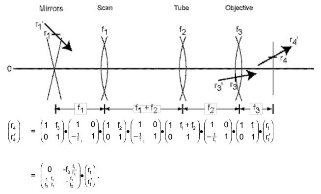
The critical point is that a change in the initial slope is turned into a change solely in position of the beam in the object plane, *i.e.*,
