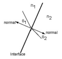
**Flat interface.** We move on to an interface with index  $n_1$  to the left and  $n_2$  to the right.
