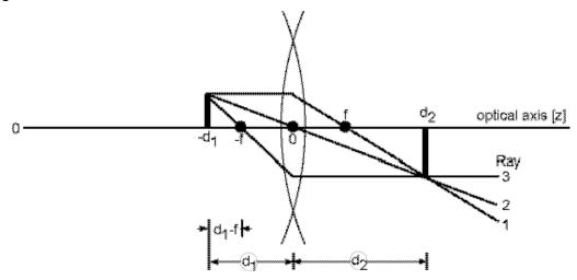
*Lens-space-lens.* A ray enters one thin lens, travels a distance d, and then exits through a second thin lens.
