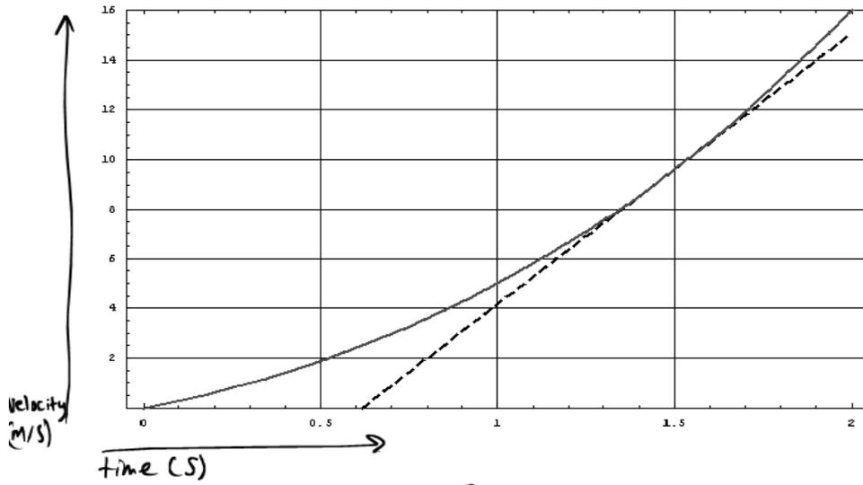
a)  $\bar{a} = \frac{\Delta v}{\Delta t} = \frac{16 \frac{m}{s}}{2.0s} = \boxed{8.0 \text{ m/s}^2}$
