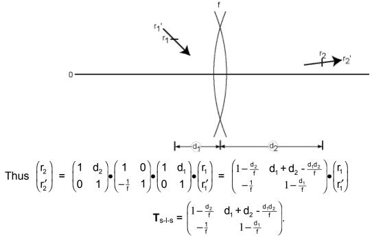
Imaging condition. This corresponds to a final height, r<sub>2</sub>, that is independent of initial slope, i.e., r'<sub>1</sub>, so that all rays that leave r<sub>1</sub> converge at r<sub>2</sub>. Thus the "B" term of the transfer matrix must be zero, i.e., d<sub>1</sub> + d<sub>2</sub> - (d<sub>1</sub>d<sub>2</sub>)/f = 0. This leads to the famous lens formula
